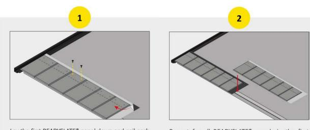
Lay the first READYSLATE® panel down and nail each piece of slate using the pre-punched holes provided. Once the panel install is complete, peel back the protective film on the top and right side of the panel.
