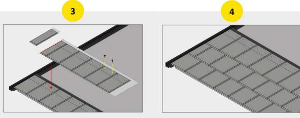
READYSLATE® is designed with an overlap line that allows for quick and easy placement of each panel.
